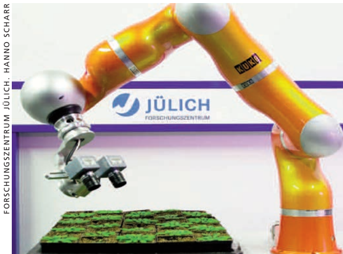
Robots are used increasingly to make real-time measurements in the laboratory and field. The GARNICS robot is designed for 3-D sensing of plant growth.
